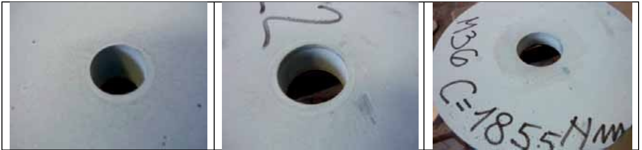
Appearance of the central perforated areas of the individual samples after compression testing by tightening the bolts.
