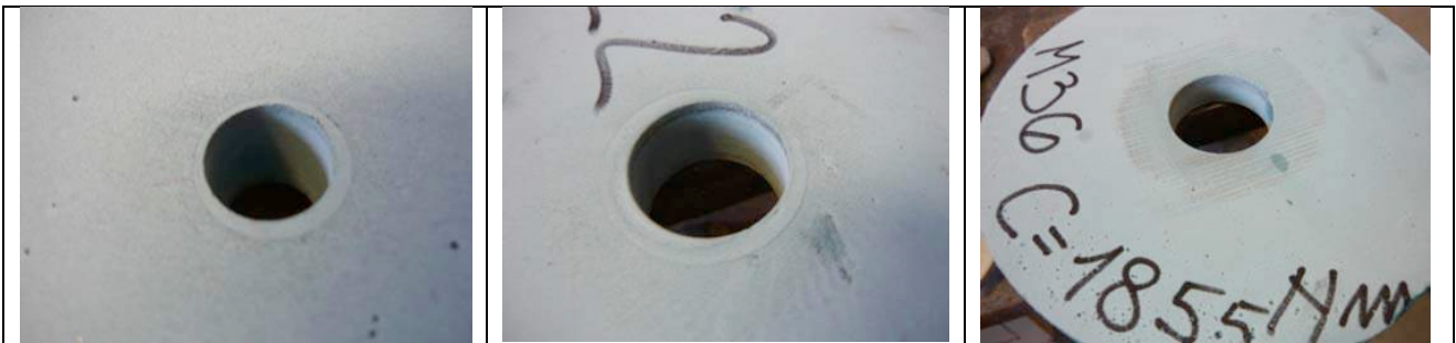
Pictures of some central area after Bolt Torque test
