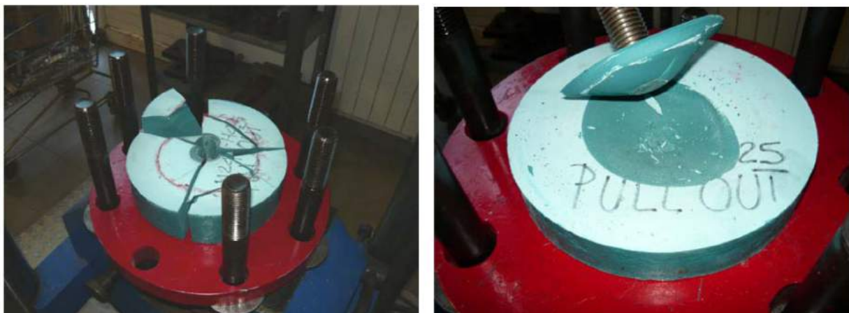
Sample M 24 - H45 and M24-H25 after the pull out test
