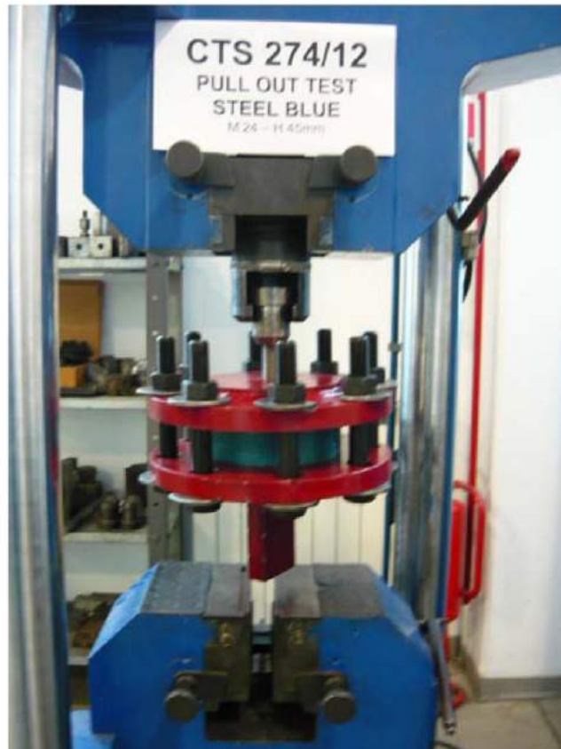
Picture of the resin sample during the pull out test (M24 – H 45mm).
